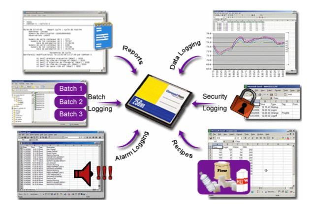
Not only does the CompactFlash interface provide expandable storage for data and event logging, it also provides a means to load the panel's database without a PC.
